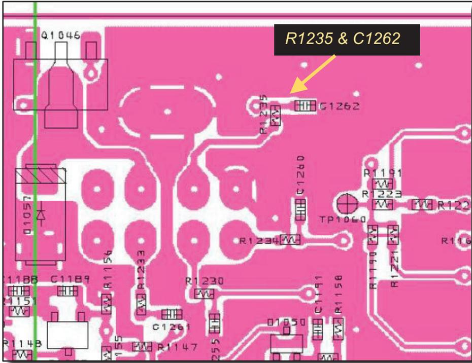
So with some trepidation the Main-Unit PCB was removed only to find that R1235 was nowhere to be found!
