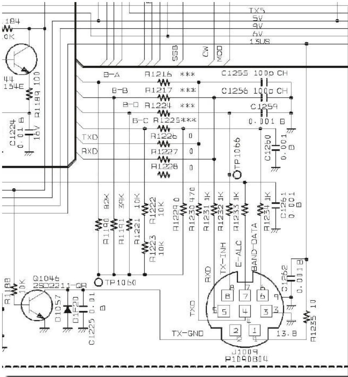
A 10 ohm R1235 resistor will provide a fairly stiff output to drive applications needing up to about 100 mA. However in measuring several transceivers it was found that the output resistance often changed with load current and varied from a high of just over 100 ohms to around 15 ohms. No method to
