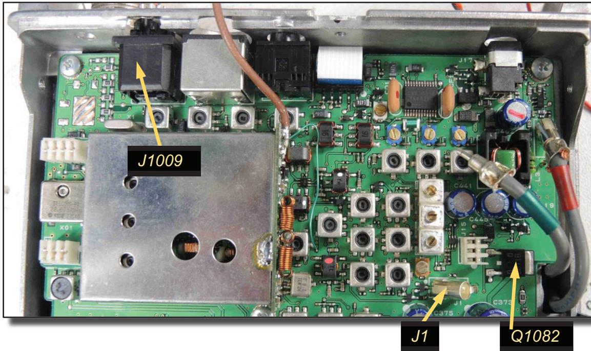
3. For convenience unplug the coax cable from the connector marked J1, (J1001 in the service manual). This makes it easier to work around Q1082. In the picture above its shown removed from J1. It's the coax shown dangling in the air with the green tape around it.
