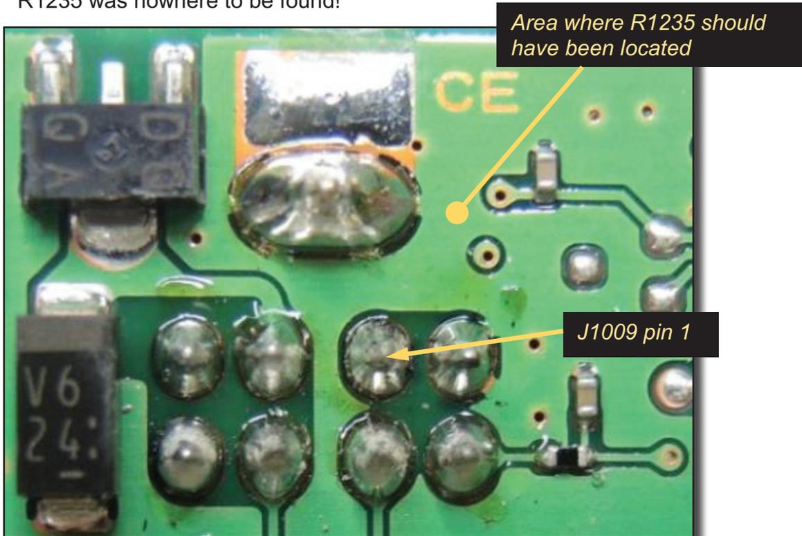
A search eventually found R1235. Yaesu had changed the printed circuit board so that the resistor is now on the top side and connects to J1009 pin 1 through a zero ohm 0805 jumper. And it's a tiny 0402 (read low power dissipation) part.
