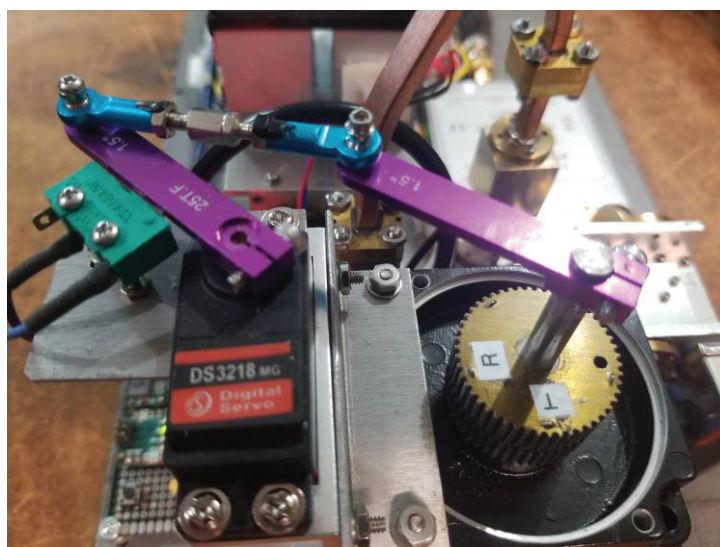
Figure 4. Waveguide switch in transmit position. Note the microswitch is closed by the arm.
