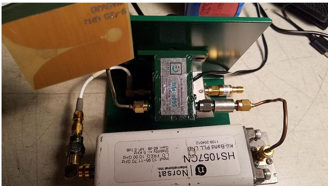
The second project was to take an L104 type of LNB and solder a piece of .085 onto the board and remove the small wire that acts as a monopole probe into the waveguide. With a very small coupling capacitor, it makes a good way to feed a coax signal into the LNB and makes a good frequency converter. It is desirable to change the crystal to a TCXO for greater stability.
