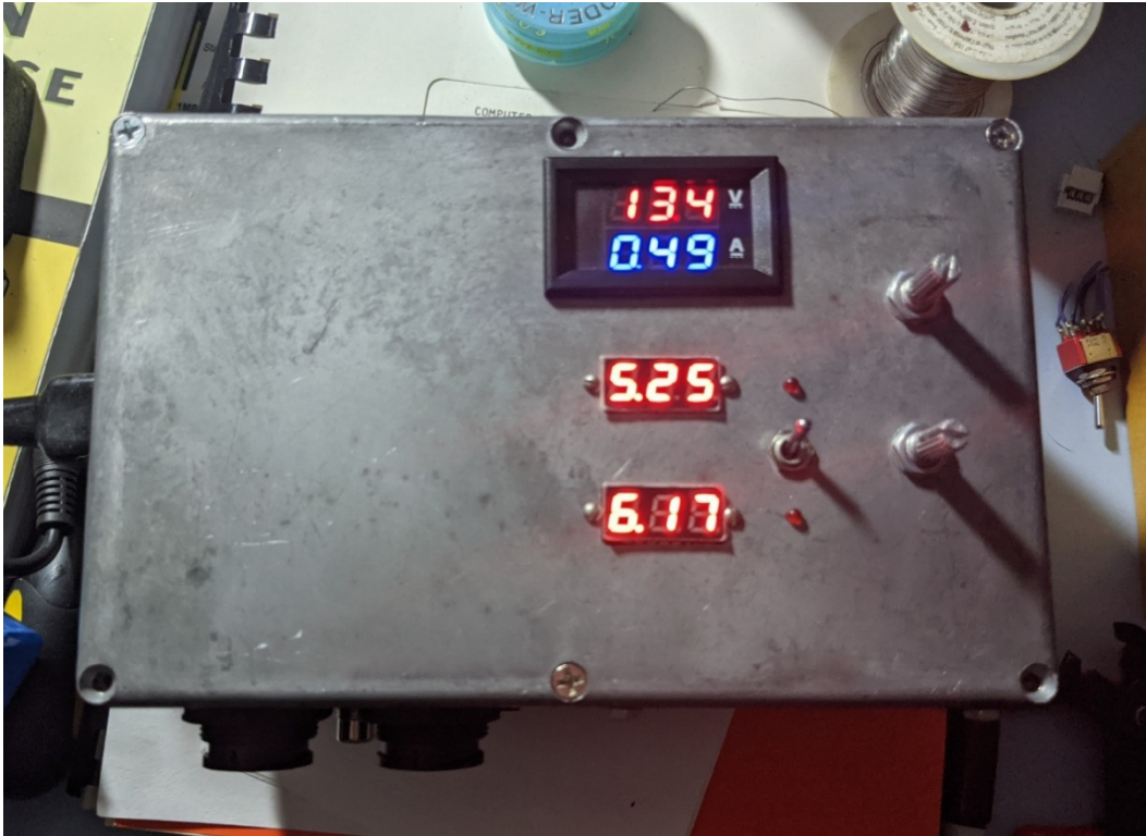
Figure 8. The photo above shows the DC subsystem in test. Total input voltage and current draw are indicated at the top while individual 5 and 6 volt meters along with trim pots are beneath and to the right.
